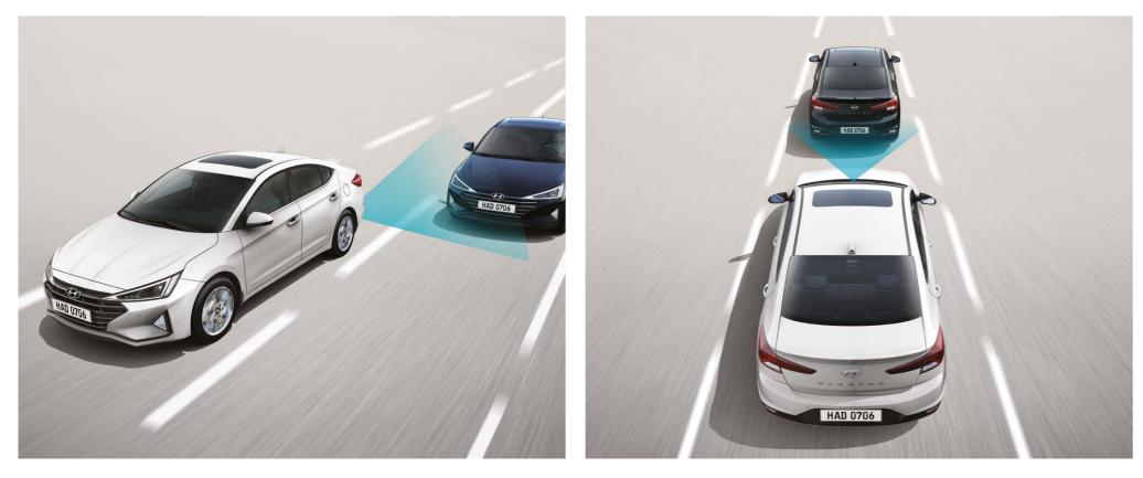
Blind-Spot Collision Warning (BCW) Reflexive radar sensors in the rear bumper warn the driver of approaching vehicles that aren't visible.
